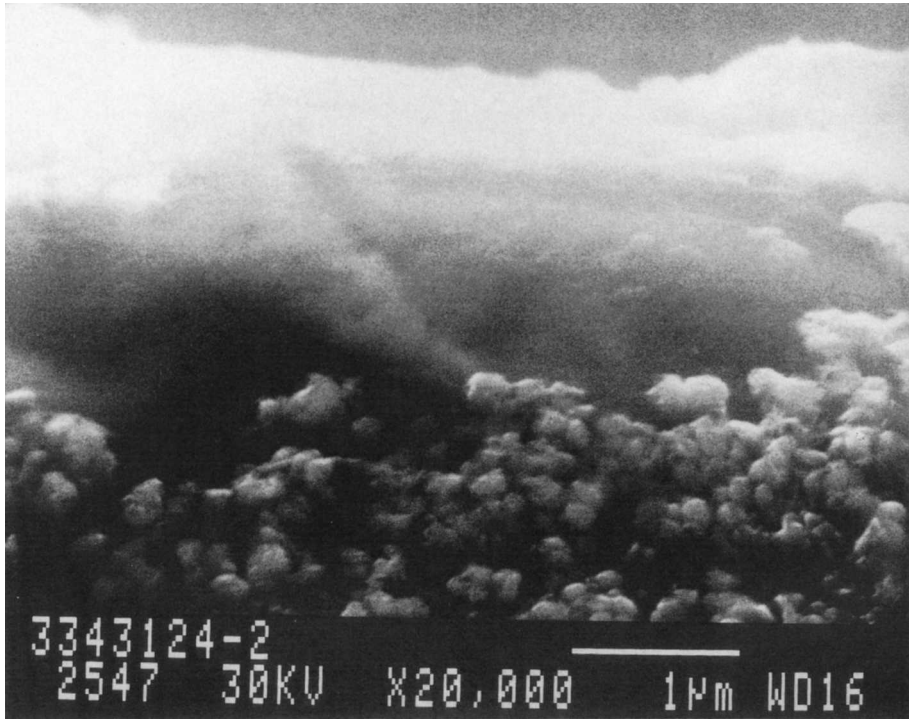
Fig. 9. SEM photomicrograph of outer edge of a cross section of a hollow fiber membrane spun from NMP : acetic acid at 20K magnification.
